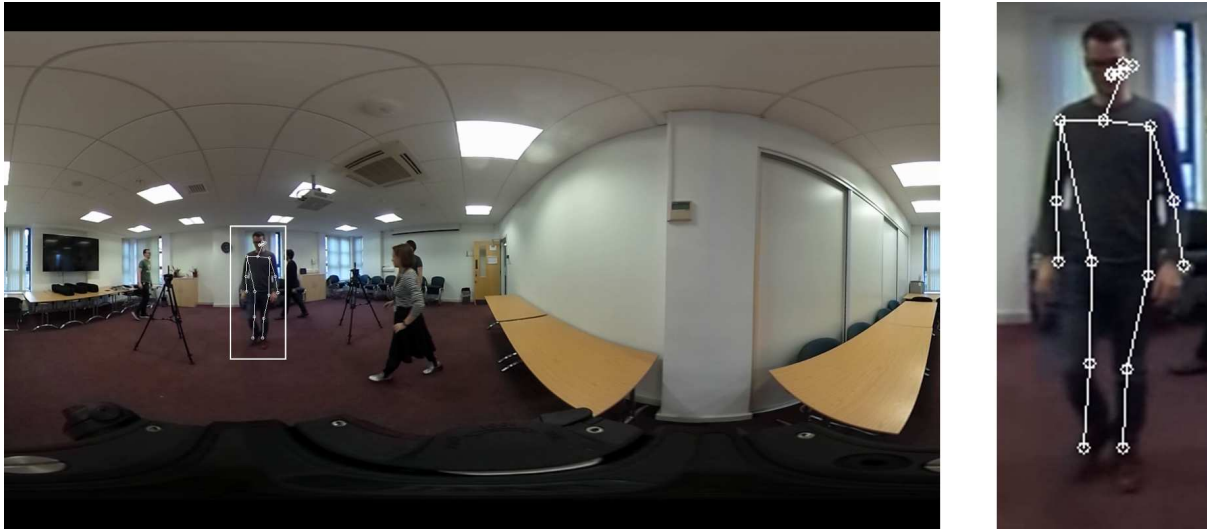
Figure 4. Example of a 3D pose estimate as viewed from the test camera, from Seminar Room
